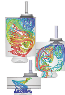
Figure 1: Transient investigation of swirling in-cylinder flow in a diesel engine Courtesy of Deutz AG
