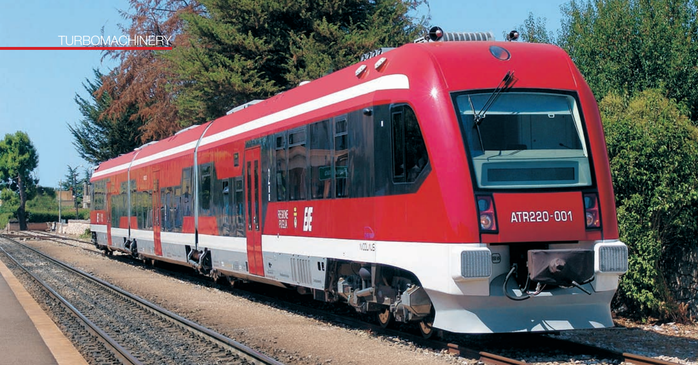
Diesel-engine ATR 220 Pesa railcar with a cooling system from Voith Turbo
